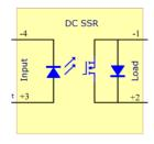
A relay completely isolates the control circuit (robotics) from the power circuit (controlled equipment), thus protecting the board and control elements.
