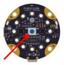
When the button is used to select options or toggle states (such as turning an LED on or off) it is convenient to include a waiting time of about 0.3 seconds since, being the processor much faster than user, as long as the user believes that performs a single press, the processor may have checked the status of the button tens or hundreds of times. Another, more efficient option is to wait for the button to be released.
