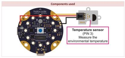
The analog temperature sensors do not directly return a value in degrees centigrade, so the gross value obtained must be processed. The TMP36 sensor, unlike thermosistors, does not use a resistance-sensitive resistor. Instead this sensor takes advantage of the property of the diodes to vary the voltage proportional to the temperature, so it is enough to read the output value and apply a rule of three.
