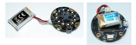
Halocode board powered by 3.7 volt LIPO batteries
