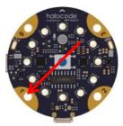
The 4 pins can be used for **digital** (ie: binary) **inputs and** outputs and for **analog outputs** (ie: values between 0 and 1023).
