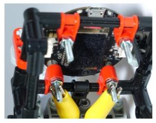
On the other hand this structure offers an adequate grip of the crocodile clips of power and ground, preventing them from making contact with other pins or components of the board, which could cause a short circuit and damage it.
