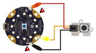
It is important to keep in mind that the crocodile clips do not make contact with each other or with other components of the board since; otherwise, it could be damaged.
