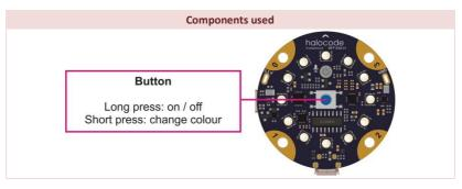
In this project we will see how to use the same component, in this case the button, to control two parameters, the status (on or off) and the color, depending on the time that is kept pressed.
