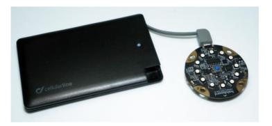
If batteries are used, they should be between 3 and 5 volts. In the market there are batteries of all sizes and capacities. For certain projects, such as
