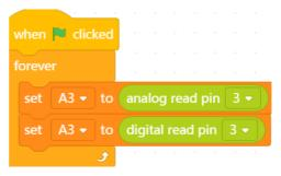
If, for example, we connect a button on pin 3 (which in principle is an analog pin), when we press it D3 will be 1 and, otherwise, it will be 0.
