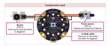
The flame sensor has a potentiometer through which you can adjust its sensitivity (left = increase sensitivity, right = reduce sensitivity).
