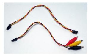
Once this change is made, the component can be directly connected to the Halocode board (G with GND, V with 3V and S with 0, 1, 2 or 3), as shown in the image.
